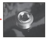
CKF2 and CKFS2 broaching-type fasteners are designed for use on printed circuit boards and on most brittle or hard materials: glass laminates, epoxy or resin with paper, nylon, or canvas bases. They are also used on materials too thin or unsuitable for threading, such as acrylic and polycarbonate panels.
